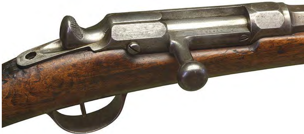
Chassepot bolt mechanism, used by French Forces 1866-1874 Invented by Antoine Alphonse Chassepot (1833-1905)
