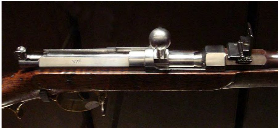
Needle Gun firing mechanism First developed in 1808
