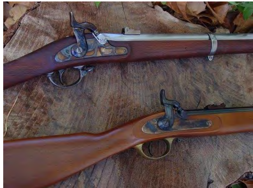
Percussion caplocks used on Springfield and Enfield rifle muskets Patented by Alexander John Forsyth in 1807
